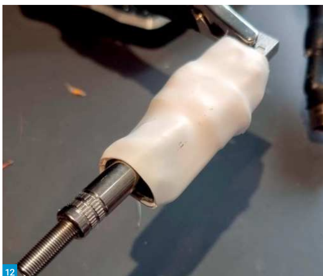
Fig. 6: Notch for the wires to pass through. Fig. 7: The debouncer circuit. Fig. 8: Physical realisation of the debouncer. Fig. 9: The completed board. Fig. 10: The board encased in hot melt glue. Fig. 11: Installing the jack socket. Fig. 12: Sealing in heatshrink. Fig. 13: The LED lights up. Fig. 14: Keyer software interface. Fig. 15: The finished project.
