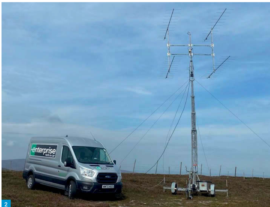
Fig. 2: Allan GM4ZUK's 2m station for the IARU 144MHz Trophy Contest. Fig. 3: An example of a DAB Slideshow from the Netherlands as received by Allan GM4ZUK. Fig. 4: The impressive 2m array at the DR9A Club station. Fig. 5: Adrian GU0VLG operating on 2m from the Guernsey Amateur Radio Society club station.
